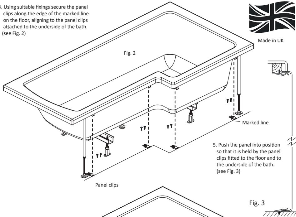
5. Push the panel into position so that it is held by the panel clips fitted to the floor and to the underside of the bath. (see Fig. 3)
